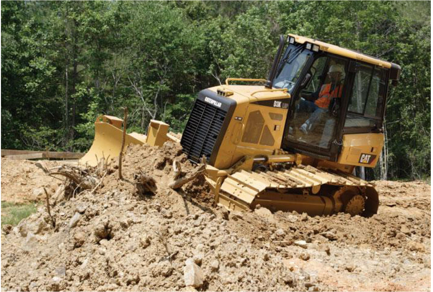
Image 4: Dozer carving a wildfire containment line. Bulldozers cause significant, long-term damage to soils, vegetation, and hydrological systems.
