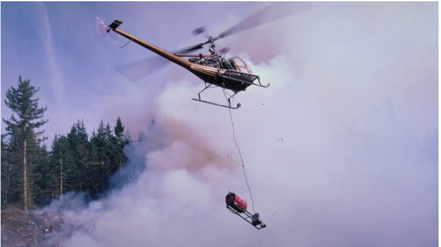
Analyzing suppression records can help determine the areas where wildfire spread advanced through backfire and burnout actions such as the use of a “helitorch” pictured above.
